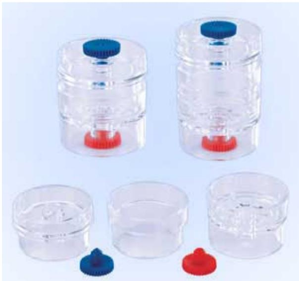
**37 mm** – Available in both a standard two-piece style and a three-piece style. These cassettes meet the NIOSH requirements for sampling most dusts, fumes and mists. Three-piece cassettes allow open face sampling, typically for asbestos and other fibers.
