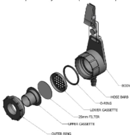
The inhalable fraction size distribution is described by the following table. For particles of 1 micron diameter, nearly all (97%) are captured by the sampler and collected onto the filter. For particles of 100 microns in diameter, 50% are collected onto the filter. This approximates the size distribution in the respiratory tract.
