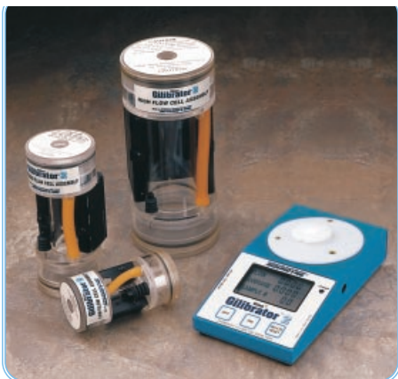
The GILBRATOR-2® Base can be used with any of three different wet cells.
