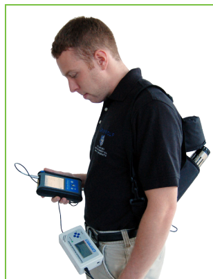
FM-80I (on included ACC-BELTCL-1 belt clip) shown connected to GrayWolf AdvancedSense
